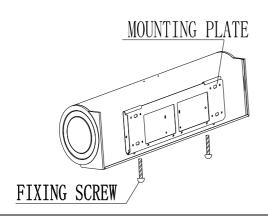
4.1.3 When the cement has freeze, fit the mounting plate (use the washer and nut according to the following)
