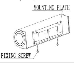
4.3.2 Fixing ceiling brackets as Fig. (optional parts) WASHER SPRING WASHER NUT
