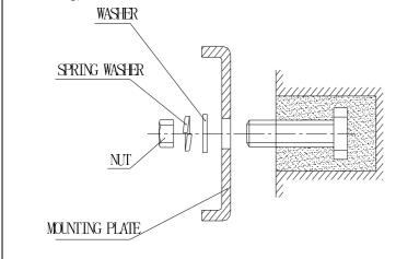
4.1.2 Fix the bolts in the proper position (Decide the position with the mounting plate and pour cement into the bolt holes.)
